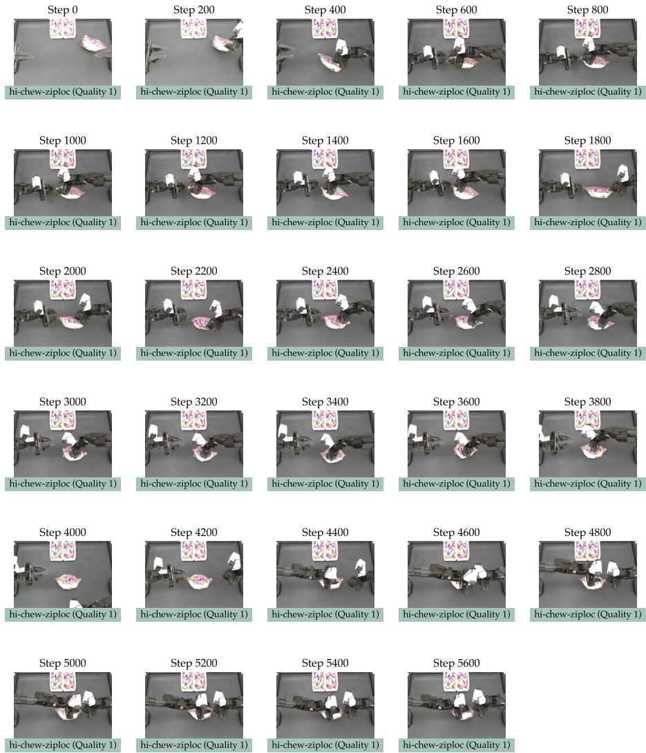
Fig. 8: In this trajectory, the user correctly moves the Ziploc from the corner of the table to the center of the table, and grasps a Hi-Chew from inside the Ziploc which they bring to the End Zone. They are unsuccessful in closing the Ziploc before episode termination. The user is task-directed for the whole episode, however takes longer than better quality trajectories for this task and performs retrying behavior at each subtask. The whole trajectory is marked as hi-chew-ziploc (Quality 1) .
